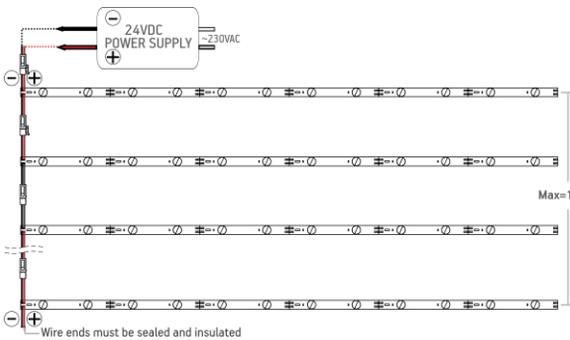
! 10 pcs - max number of LED bars in one chain when the power supplied from single end.
