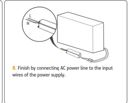
\*Take in consideration the insulation class for the power supply and connectors outside the lightbox, depending on the place it will be stored.
