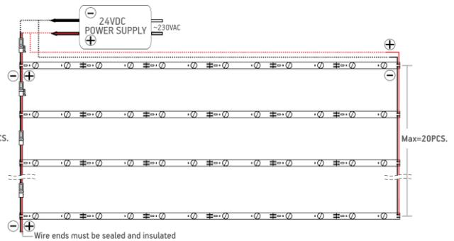
! 20 pcs - max number of LED bars in one chain when the power supplied from both ends (additional wiring is needed)
