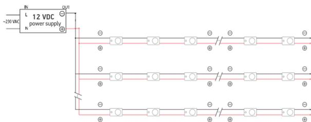
! 24 pcs - max number of modules in one chain when the power supplied from single end.
