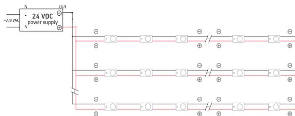
! 66 pcs - max number of modules in one chain when the power supplied from single end.
