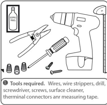
1 Tools required. Wires, wire strippers, drill, screwdriver, screws, surface cleaner, terminal connectors and measuring tape.
