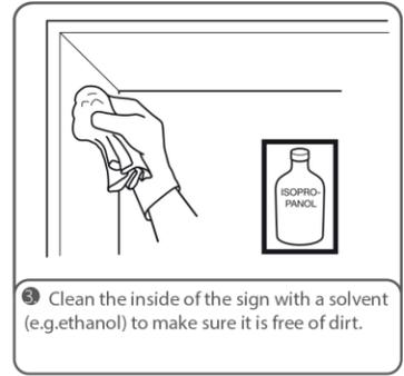
3 Clean the inside of the sign with a solvent (e.g. ethanol) to make sure it is free of dirt.
