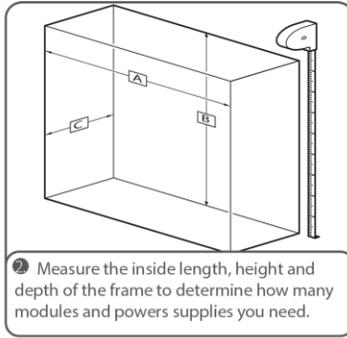
2 Measure the inside length, height and depth of the frame to determine how many modules and power supplies you need.
