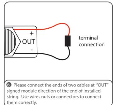
6 Please connect the ends of two cables at "OUT" signed module direction of the end of installed string. Use wire nuts or connectors to connect them correctly.
