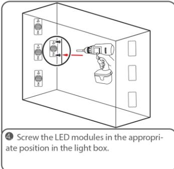
4 Screw the LED modules in the appropriate position in the light box.
