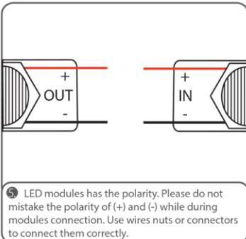
5 LED modules has the polarity. Please do not mistake the polarity of (+) and (-) while during modules connection. Use wire nuts or connectors to connect them correctly.
