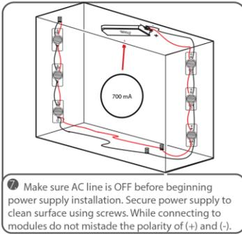
7 Make sure AC line is OFF before beginning power supply installation. Secure power supply to clean surface using screws. While connecting to modules do not mistake the polarity of (+) and (-).
