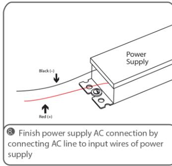
8 Finish power supply AC connection by connecting AC line to input wires of power supply
