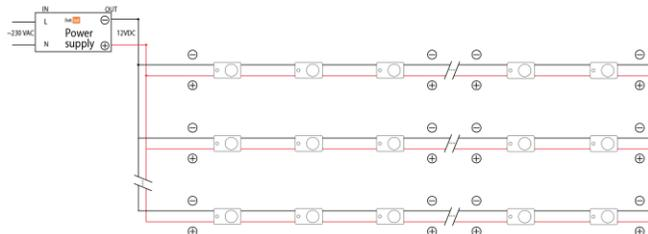
! 50 pcs - max number of modules in one chain when the power supplied from single end.
