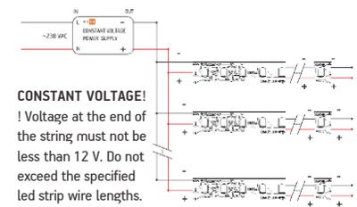
**! Only PWM dimming is suitable for LineLit ZigZag.**
