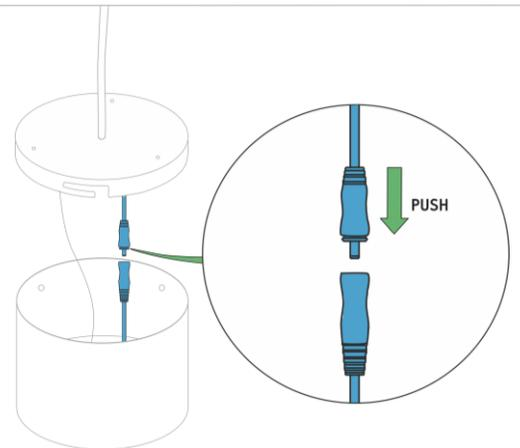
6 Connect DC connector between driver and luminaire.
