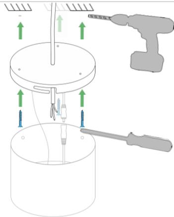
3 Fix the back plate onto the ceiling with 3 screws.
