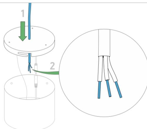
2 Bring power cable front of back plate by using hole in the middle. Strip the wires.
