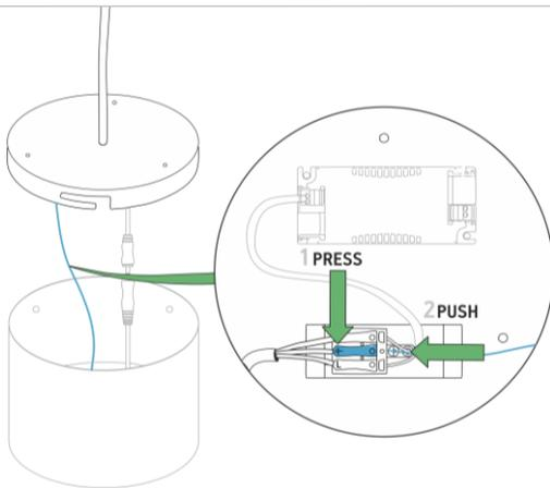
5 Fix secure wire to the ground hole at grounded terminal block.
