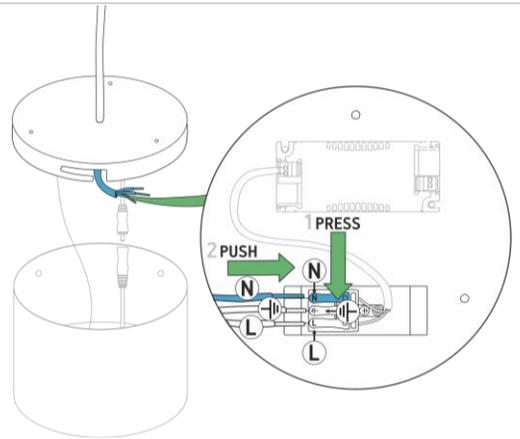
4 Connect power cable to grounded terminal block. Push each terminal's pin while putting in the wires to appropriate terminal block's line.
