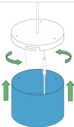
7 Install luminaire to back plate and twist to fix.
