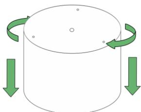
1 Separate luminaire from back plate by twisting it.
