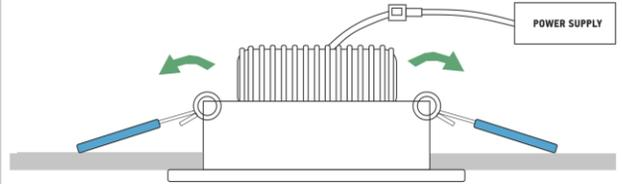
4 Once LED downlight is in the hole the lugs will come down and light will be secured
