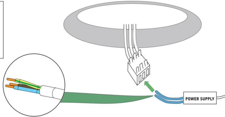
2 Strip the wires and connect them with the power supply.
