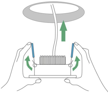
3 Push up the two lugs on the Heronlux and then push the light up into the hole.
