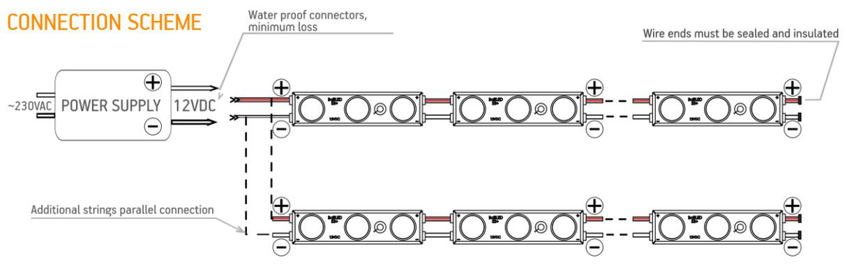
! 35 pcs - max number of modules in one chain when the power supplied from single end.
