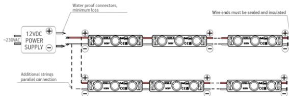
! 20 pcs - max number of modules in one chain when the power supplied from single end. ! String end voltage can't be less than 11V, do not exceed specified module string length
